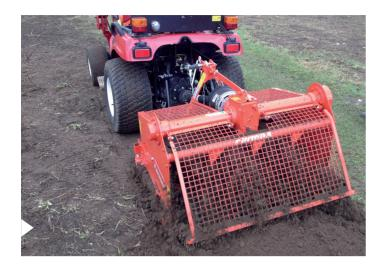
Drive: Single-sided chain transmission Tractor power: 20 to 35 HP Power take-off revs: 540 r.p.m.
