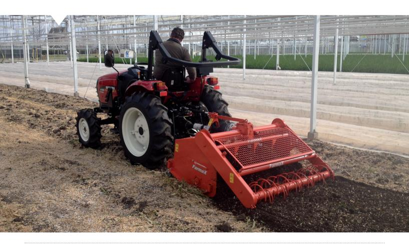
The Farmax ERP is a spader for light tractors. The great manoeuvrability and low integral weight of the ERP make it highly suitable for use in greenhouse horticulture, flower cultivation and tilling small plots.
